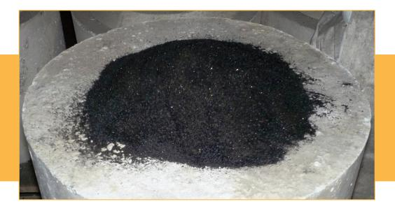
FRC Global offers a variety of Flosan® products, customizable for your operation and needs. Each blend is intended to optimize free-open performance under your unique conditions. While the majority of the product is used as ladle nozzle fill in ladle sliding gate systems, it has been used in E.B.T. furnace tapholes.
